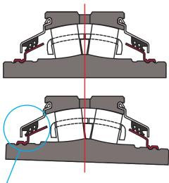
Positive seal contact is maintained during mis-alignment at any angle.
