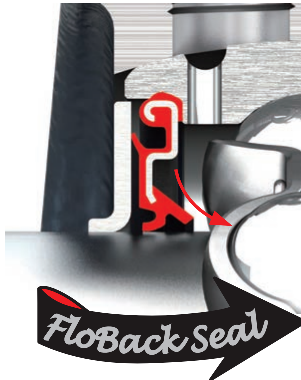
Fig. 1.3 Sealing mechanism of ball bearing units
