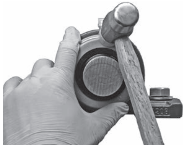
Fig. 14.14 Installing steel plate covers
