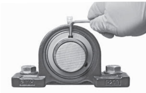
Fig. 14.5 Tightening of set screws
